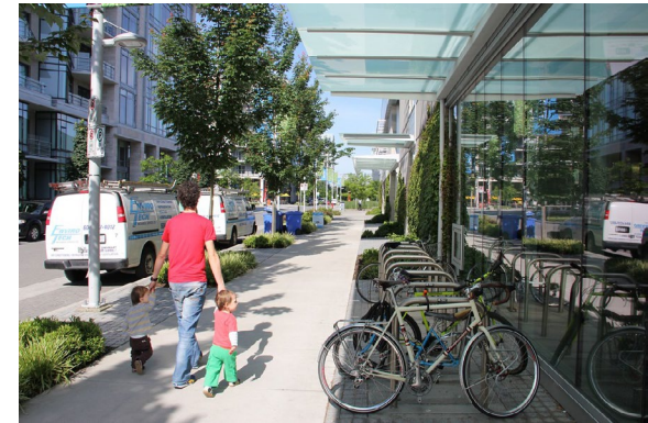
Figure 18: Benches and bike racks should be located to one side of accessible pathways (3.7.f).
