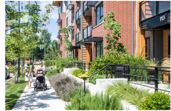
Figure 29: Set back residential buildings on the ground floor between 4-6 m to create a semi-private entry or transition zone (4.2.g).
